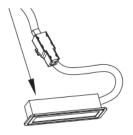
4. Open the protection cover as shown in the picture below and unplug the connected plastic shell to replace with a new lamp.
